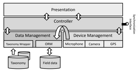
Fig. 1. Four-tier architecture of DiversityMobile
